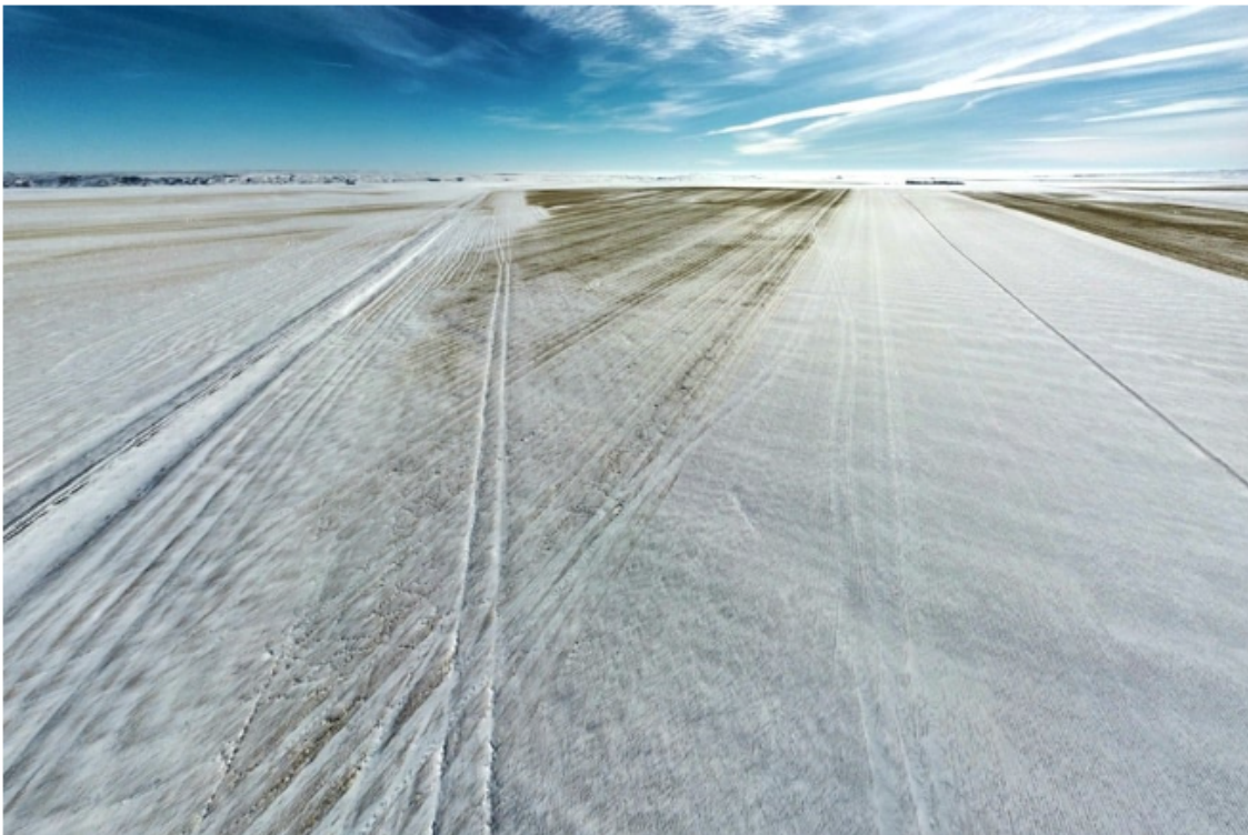
A drone image, taken by Dr. Philip Harder, then with the University of Saskatchewan's Centre for Hydrology, shows the test field in February 2023 with different amounts of snow trapped by different stubble heights.
